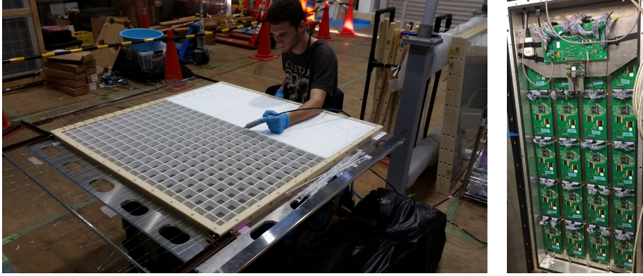
Figure 13: Left panel shows the assembly of the 3D scintillator grid. Right panel shows the DAQ of one WAGASCI module, developed at LLR starting from the SiWecal acquisition system, with 20 ASU cards treating the signal from 32 MPPC.
