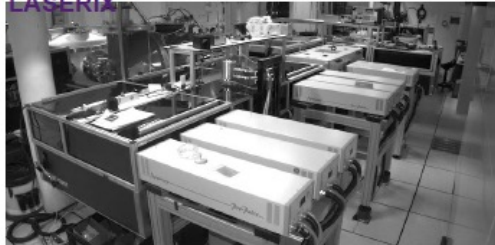
40 TW, 10Hz laser driver system, LASERIX
