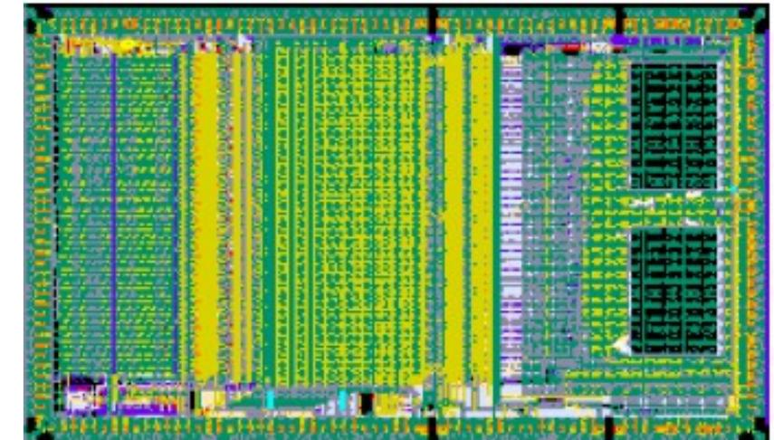
64 Channels with three thresholds
