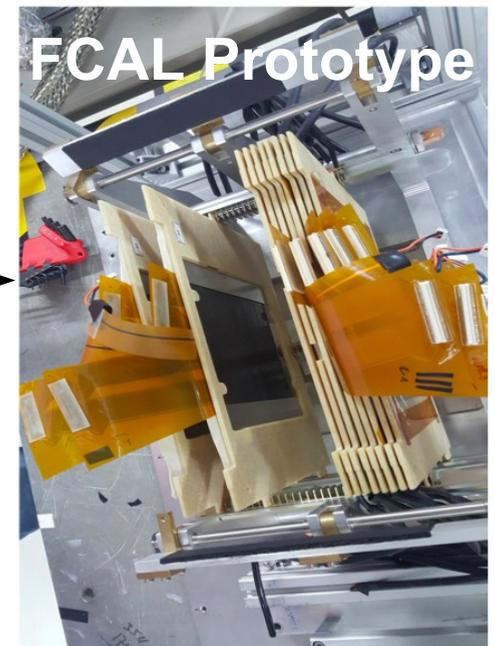
Adaptation of compact readout system developed for SiW ECALs to other prototypes of granular calorimeters
