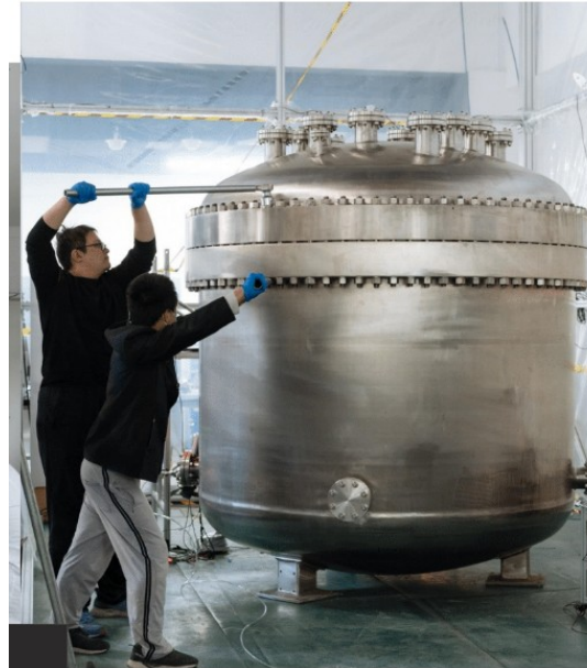
TPC vessel produced, production of shielding ongoing
