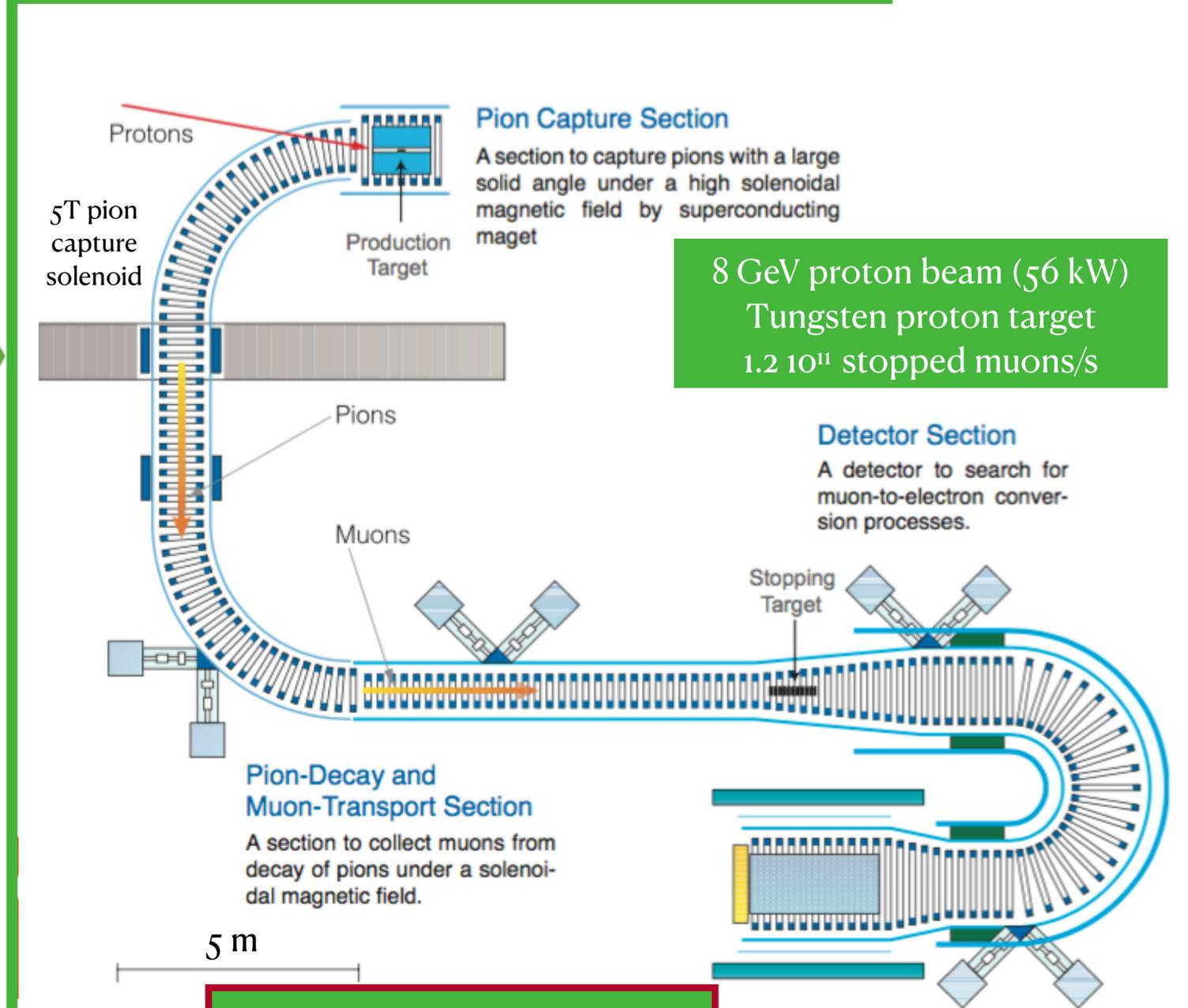
8 GeV proton beam (56 kW)
