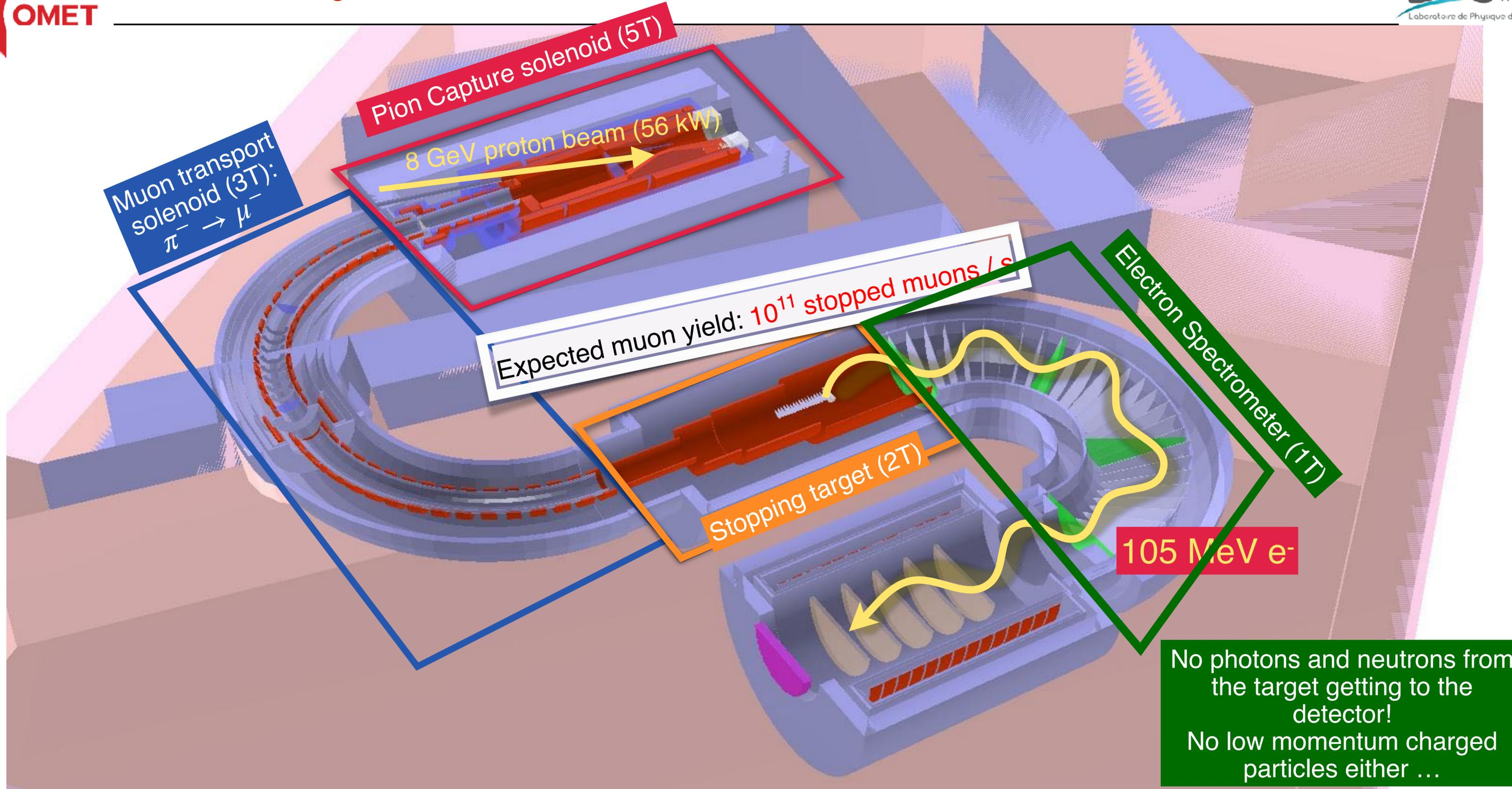
No photons and neutrons from the target getting to the detector!
