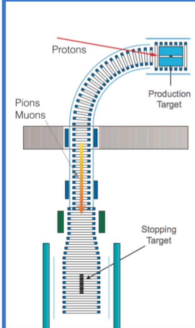
8 GeV proton beam (3.2 kW)
