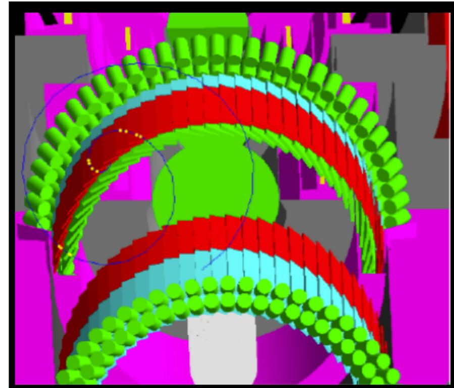
2-rings of ultra fast scintillators (64 segments, 33/36 x 1 x 1 cm<sup>3</sup>) read by optical fibres and SiPMs
