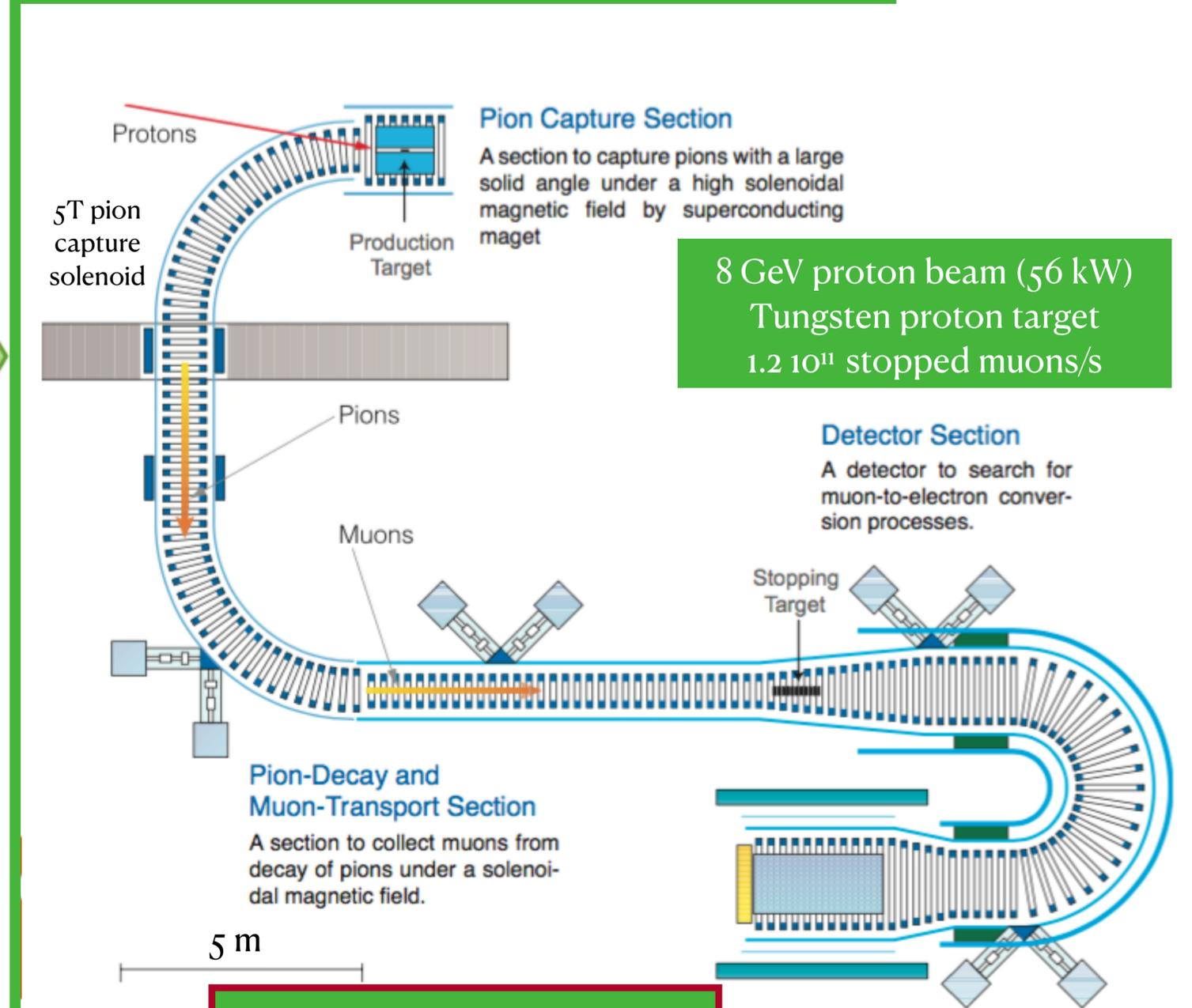
8 GeV proton beam (56 kW)
