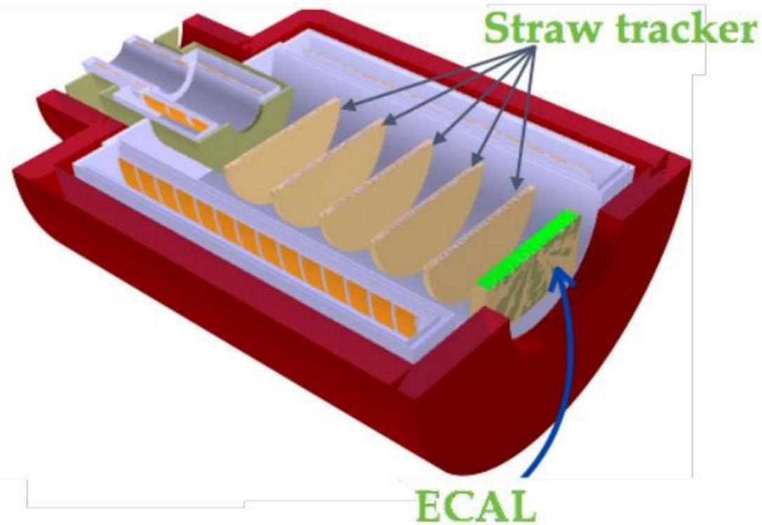
5 stations of straw detectors+ ~2000 LYSO-cells calorimeter
