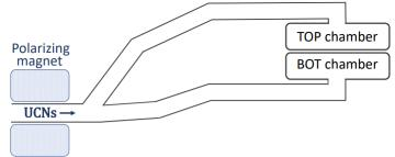
(a) Polarized UCNs fill the precession chambers
