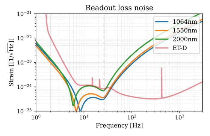
The SRC is detuned to give identical optical resonant frequency. 92% PD efficiency is assumed for 2000nm.
