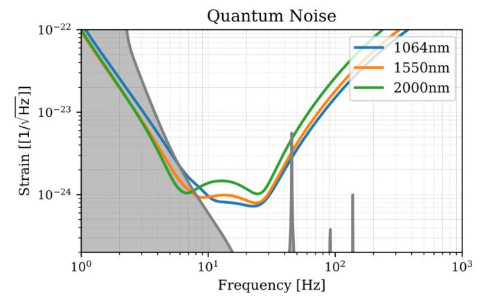
The sum of seismic, Newtonian and suspension thermal noise@10K is set to be the low frequency barrier.
