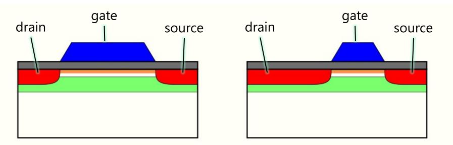
reduce gate length to minimize the internal gate and increase charge gain
