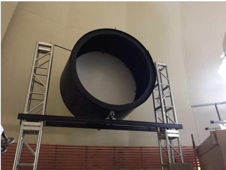
Flat-field illuminator (32 pulsed LEDs per colour)
