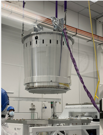
Cryostat being installed in the tip-tilt fixture
