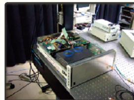
Portable optical frequency comb
