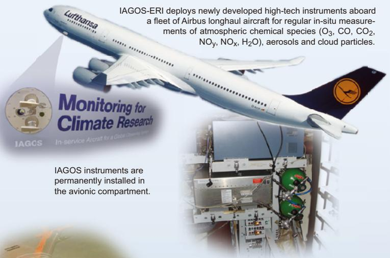
IAGOS-ERI deploys newly developed high-tech instruments aboard a fleet of Airbus longhaul aircraft for regular in-situ measurements of atmospheric chemical species (O<sub>3</sub>, CO, CO<sub>2</sub>, NO<sub>y</sub>, NO<sub>x</sub>, H<sub>2</sub>O), aerosols and cloud particles.
