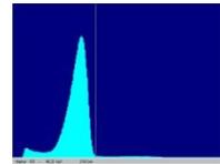
Fig. 7 X-ray spectrum of full power test with 26 MHz RF power source without beam
