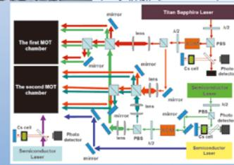
Fig. 7 Laser system for double MOT and optical pumping.
