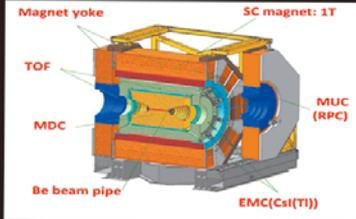
**BESIII: a large solid-angle magnetic spectrometer at Beijing Electron-Positron Collider (BEPC) for studies of Tau-charm physics.**
