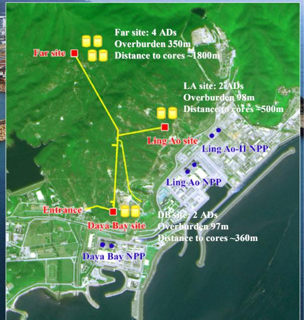
Near-far relative measurement greatly reduces systematic errors. Identical ADs will be put at 3 sites, which are connected by horizontal tunnel in the mountains.
