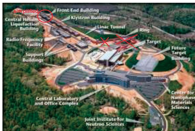
Compared to the conventional short pulse spallation sources, here SNS, Oak Ridge, USA, the Long Pulse concept of ESS offers a simplified accelerator system:  $H^+$  linear accelerator without accumulator ring reduces technical challenges (injection, space charge, target fatigue) and offers superior neutron beam performance by more neutrons /pulse.
