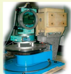
Mainly studying the texture in the industrial materials such as deep-drawing materials, shape memory alloy, tyre wires and second generation high-temperature superconducting wires.
