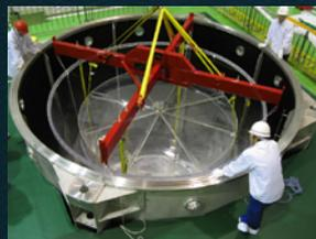
Antineutrino Detector (AD) is a 5mX5m cylinder, filled with 3 different liquids separated by acrylic vessels (AV). Gadolinium-doped liquid scintillator (Gd-LS) is used as neutrino target. Each AD weighs ~110 ton.
