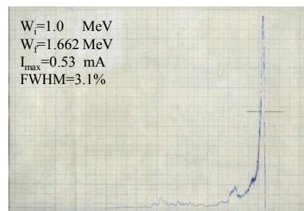
Fig. 9 Output Energy Spectrum of the  $O^+$  beam
