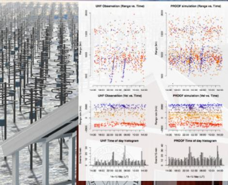
Space debris detected using the EISCAT UHF system on May 14-15th 2009, a few months after the Iridium-Cosmos satellite collision. The Iridium cloud orbital plane passes are visible at about 00:00 and 13:00 UT; and the Cosmos cloud pass at about 00:00 and 06:00 UT. The figure also compares the measurement with a statistical debris model called PROOF.
