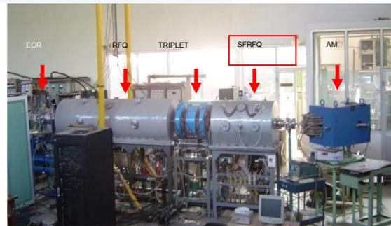
Fig. 8 The Layout of the SFRFQ beam test
