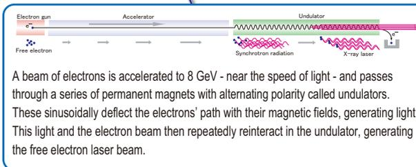
A beam of electrons is accelerated to 8 GeV - near the speed of light - and passes through a series of permanent magnets with alternating polarity called undulators. These sinusoidally deflect the electrons' path with their magnetic fields, generating light. This light and the electron beam then repeatedly reinteract in the undulator, generating the free electron laser beam.
