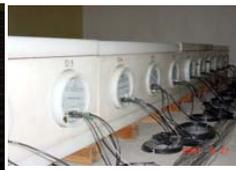
Multi-directional muon telescope and sandwich neutron system (IHEP)
