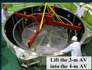
Antineutrino Detector (AD) is a 5mX5m cylinder, filled with 3 different liquids separated by acrylic vessels (AV). Gadolinium-doped liquid scintillator (Gd-LS) is used as antineutrino target. Each AD weighs ~110 ton.
