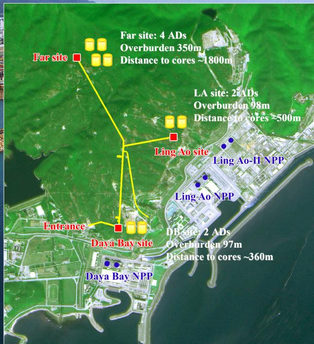
Near-far relative measurement greatly reduces systematic errors. Identical ADs will be put at 3 sites, which are connected by horizontal tunnel in the mountains.
