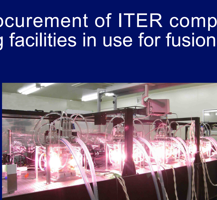
Diagnostics Test Facility Developing a high-energy-output (5 J) and high-repetition-rate (100 Hz) YAG laser for edge Thomson scattering system.
