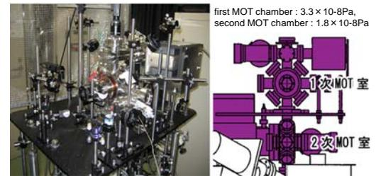
Fig. 7 Laser system for double MOT and optical pumping.
