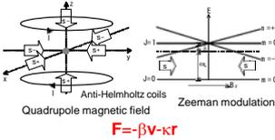
Fig. 3 Principle of the magneto-optical trapping in the two level system.
