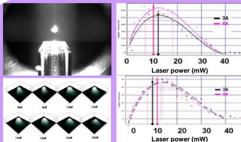
Fig. 8 Luminescence of cold Cs atoms trapped in the 1-st MOT observed by the infrared sensitive CCD camera(upper left), and their intensity profiles depending on the cooling laser power(lower left). Laser power dependences of total number of atoms trapped(upper right) and number density(lower right) in arbitrary units.
