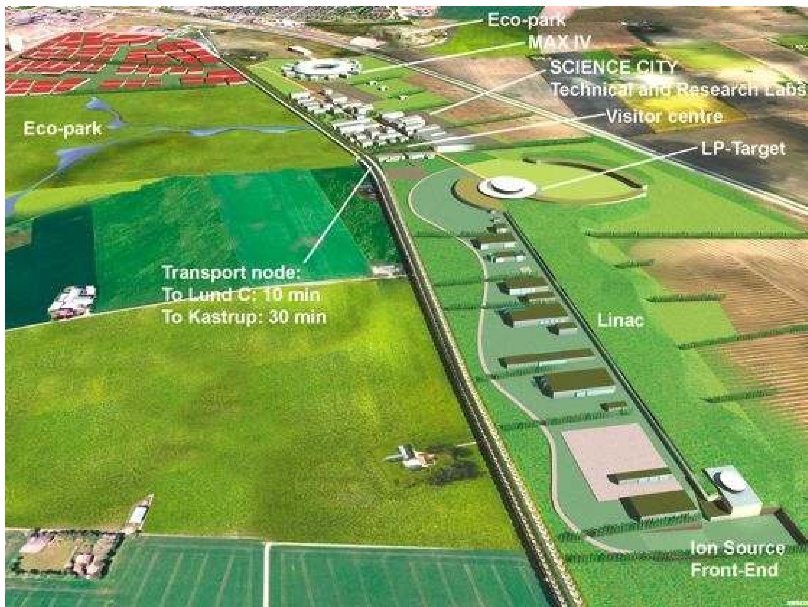
Artists' conception of ESS on a green field site outside the university town Lund. It will consist of a linear proton accelerator, a target station as the neutron beam source and a host of neutron scattering instruments at 15 – 100 m distance from the target.
