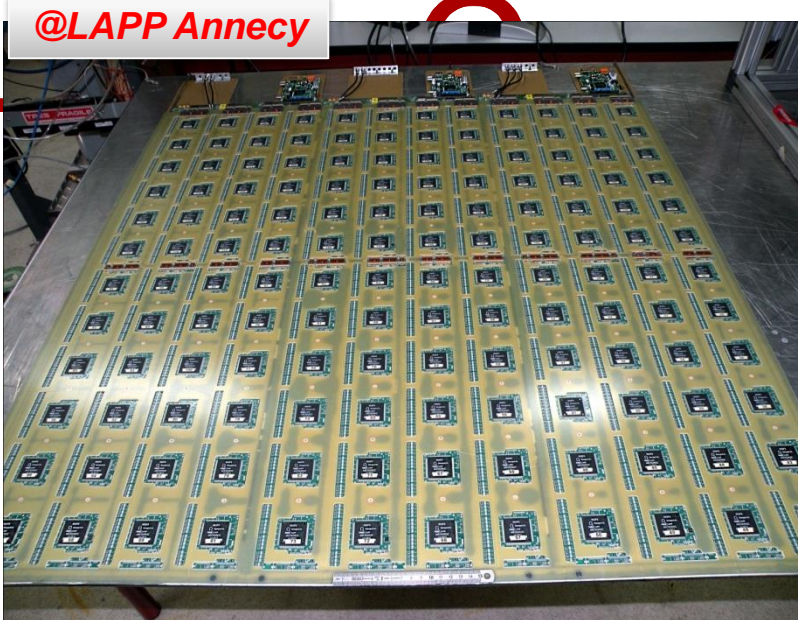
1m 2 Micromegas detector 144 Microroc : 10 000 channels
