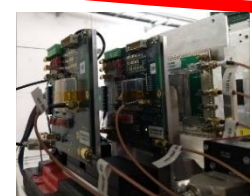
Figure 4.10: Seven 8" silicon sensor modules, equipped with SKIROC2_CMS ASIC, mounted on a copper support/cooling plate during the 2017 testbeam campaign.
