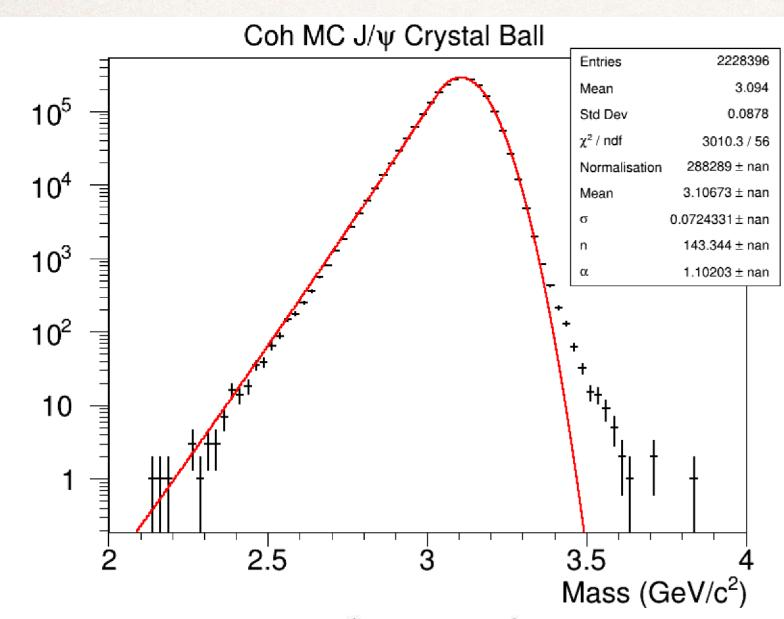
$$f(x;lpha,n,ar{x},\sigma)=N\cdot egin{cases} \exp(-rac{(x-ar{x})^2}{2\sigma^2}), & ext{for } rac{x-ar{x}}{\sigma}>-lpha \ A\cdot(B-rac{x-ar{x}}{\sigma})^{-n}, & ext{for } rac{x-ar{x}}{\sigma}\leqslant-lpha \end{cases}$$
