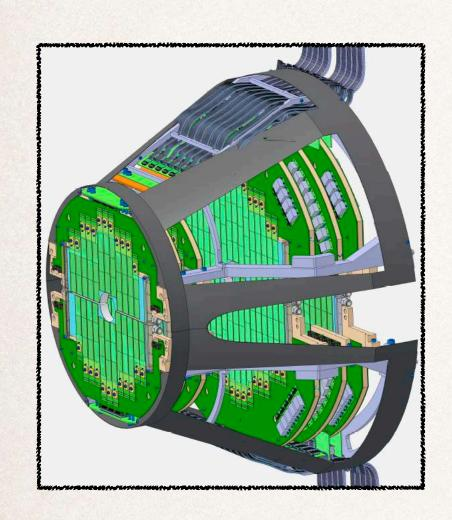
**Type of detector:** internal all-silicon-pixel tracker which will give a precise determination of the muon production vertex.
