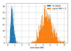
Estimated signal SNR for noise-only inputs and for  $\emph{SNR}=5$  inputs.
