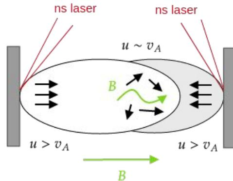
The magnetic field  $B \sim 0.5$  MG (50 T) can be produced with Helmholtz coils on  $\sim \text{cm}^3$  [Albertazzi+ 2013]
