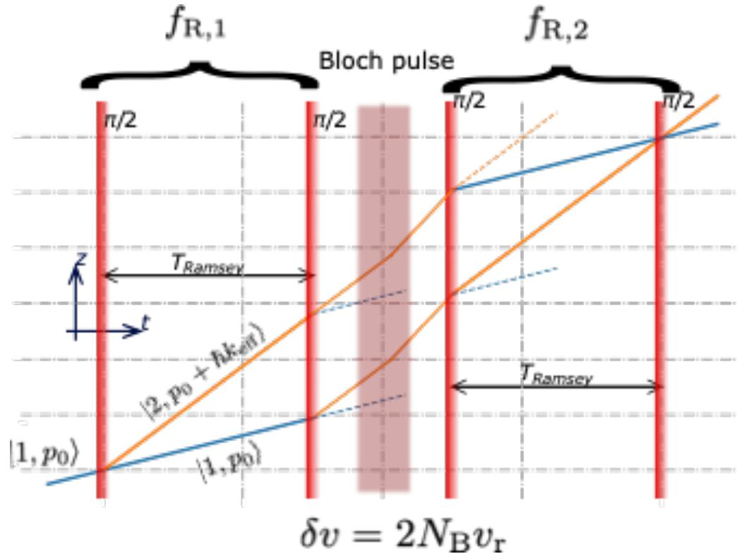
$$\Delta\Phi = T_{\text{Ramsey}} (2N_B k_R v_r - 2\pi\delta f_R)$$
