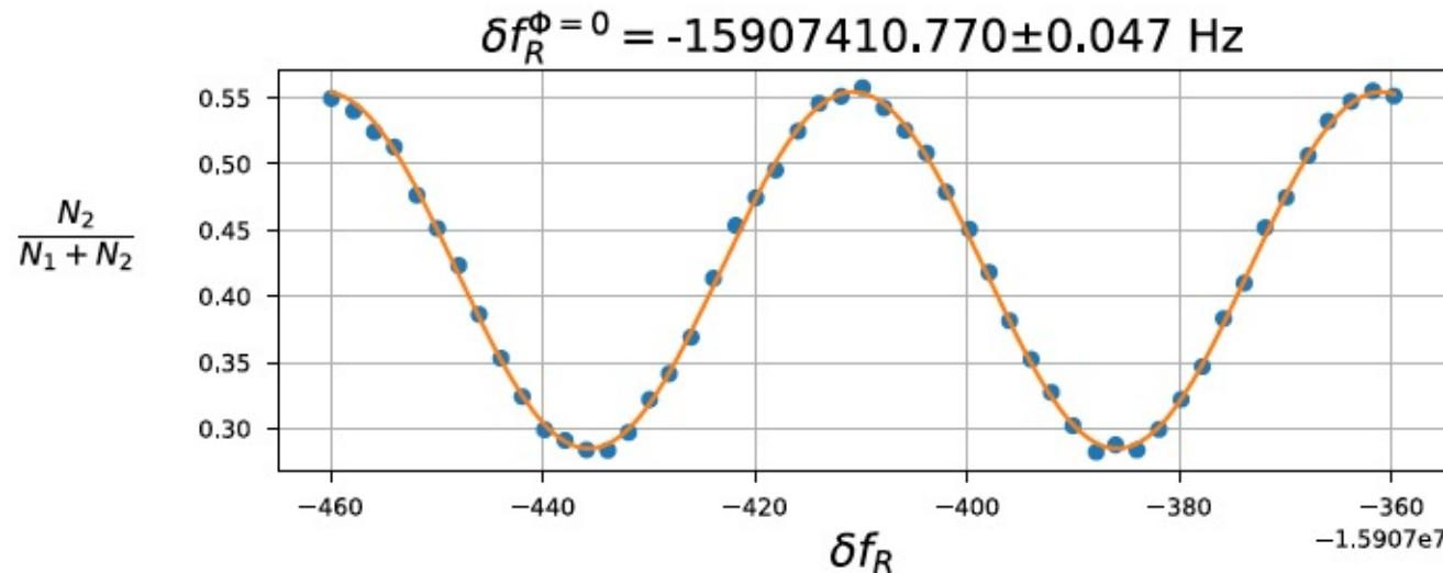
$$\Phi = T_{\text{Ramsey}} \left( k_R \left( 2N_B \frac{\hbar}{m} k_B - gT \right) - 2\pi\delta f_R \right) + \Phi^{LS}$$
