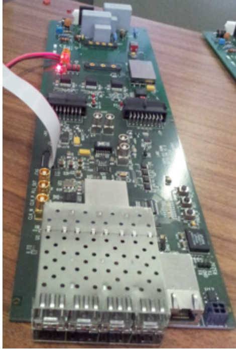
Figure 17: The custom board proposed as Time Distribution Module prototype to implement the custom distribution scheme. The design can be easily modified to host more optical ser-des.
