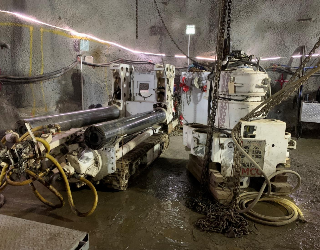
Raise Bore Machine being assembled in 3650L cavern
