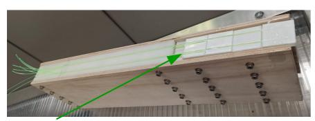
**WLS** collecting light from each module through grooves on the frontal face of scintillator tiles
