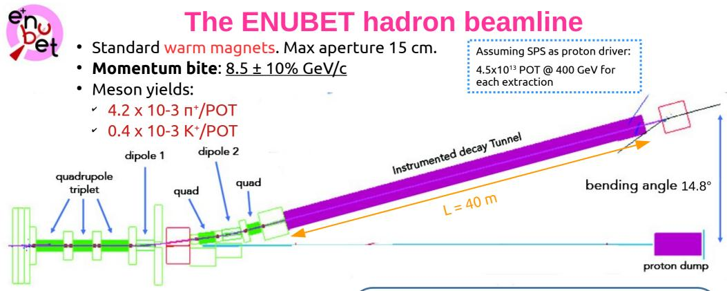
Collimators and shieldings tuned to keep under control backgrounds in the tunnel while retaining large enough meson yields
