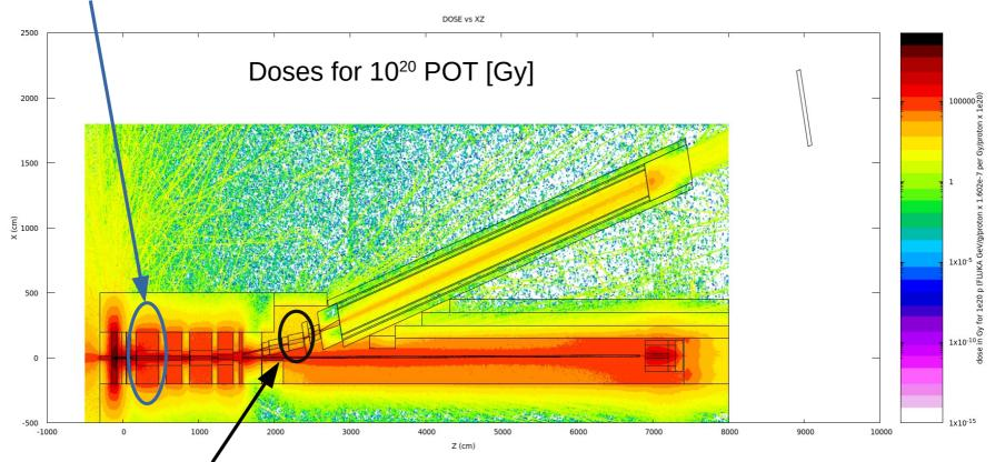
Doses at the second dipole could allow to place a **Super Conducting magnet**:
