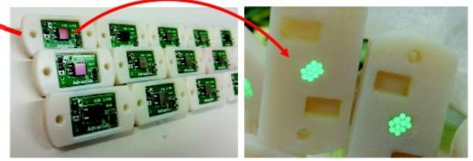
SiPM installed outside calorimeter, above shielding: reduce neutron radiation damage
