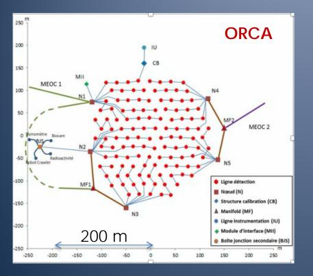
1 builing block (115 detection units) 18 DOMs / DU inter-DU distance: 20 m inter-DOM distance: 9 m
