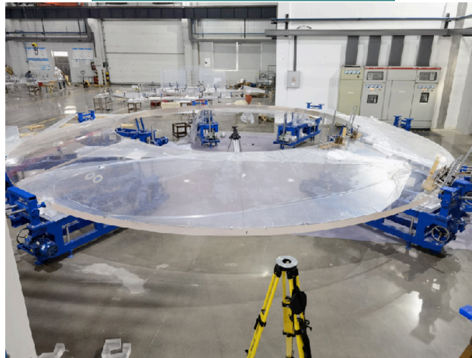
Acrylic panel assembly test
