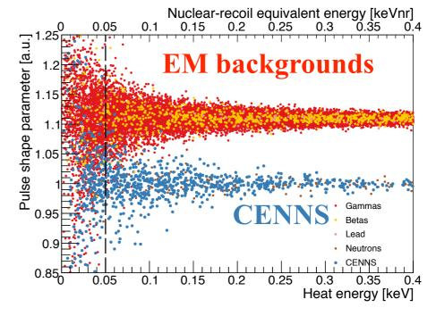
Particle ID based on Prompt / delayed heat signals
