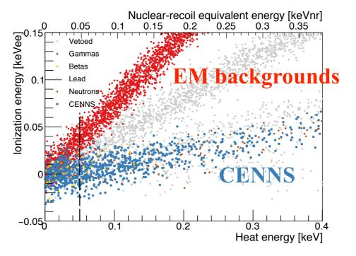
Particle ID based on **Ionization** / **heat** ratio JINR-IN2P3 meeting
