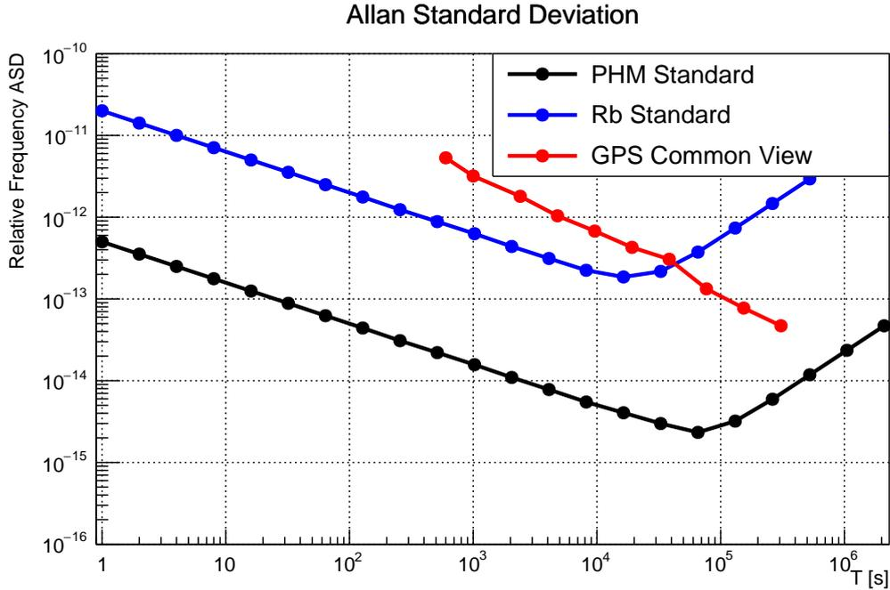
Figure 3: Relative frequency Allan Standard Deviation of the two selected clock generation systems and the GPS Single View [2].
