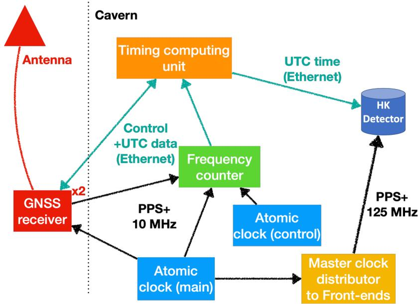
Figure 2: Detailed scheme of the clock generation section.
