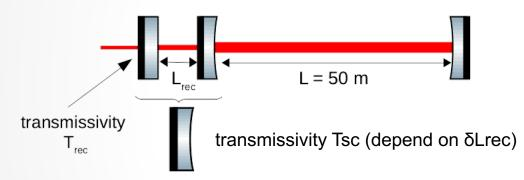
Simulation on-going to determine the optimal parameters for the coupled cavity (reflectivities, mirrors radius of curvature, etc.)
