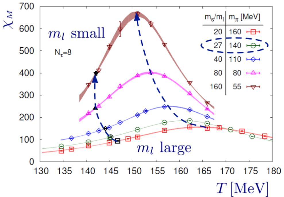
Chiral susceptibility:  $\chi_M \propto \frac{\partial \langle \bar{\psi} \psi \rangle}{\partial m_l} \sim m_l^{1/\delta-1} f_\chi(z)$ ,  $z \equiv t m_l^{-1/\beta\delta}$
