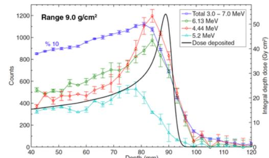
From Verburg et al., "Energy- and time-resolved detection of prompt gamma-rays for proton range verification", Phys. Med. Biol. (2013).
