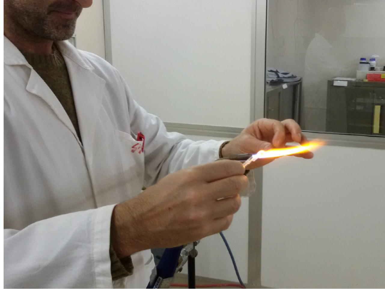
Preparation of standards inside quartz vials (for high neutron fluxes)
