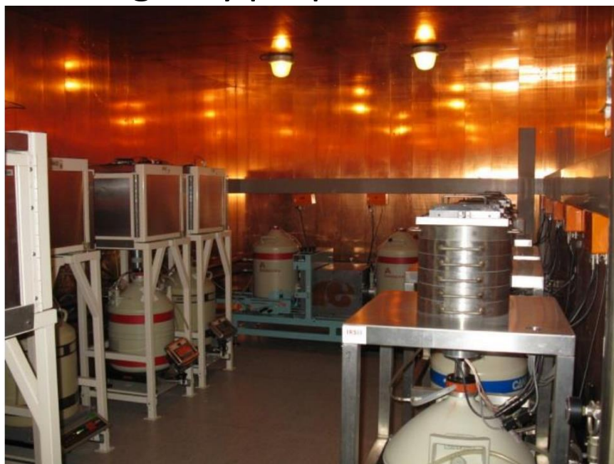
HPGe detectors in Orsay : the inner layer of the shielding covering the walls can be seen
