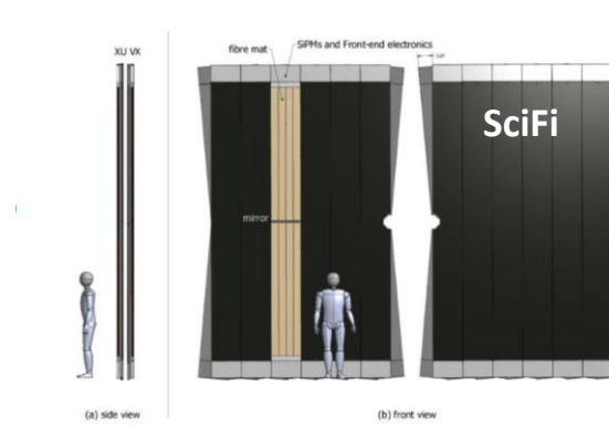
Layout of one of three stations for the LHCb SciFi Tracker.
