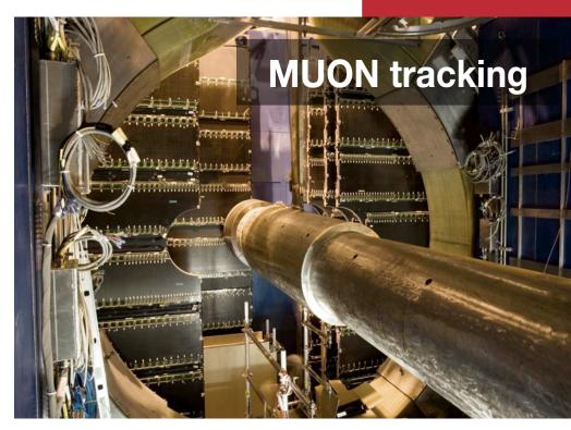
Electronics and readout being upgraded within ALICE Upgrade during LS2 (up until next year) MCH needs to be commissioned (installation and quality control of the detectors)
