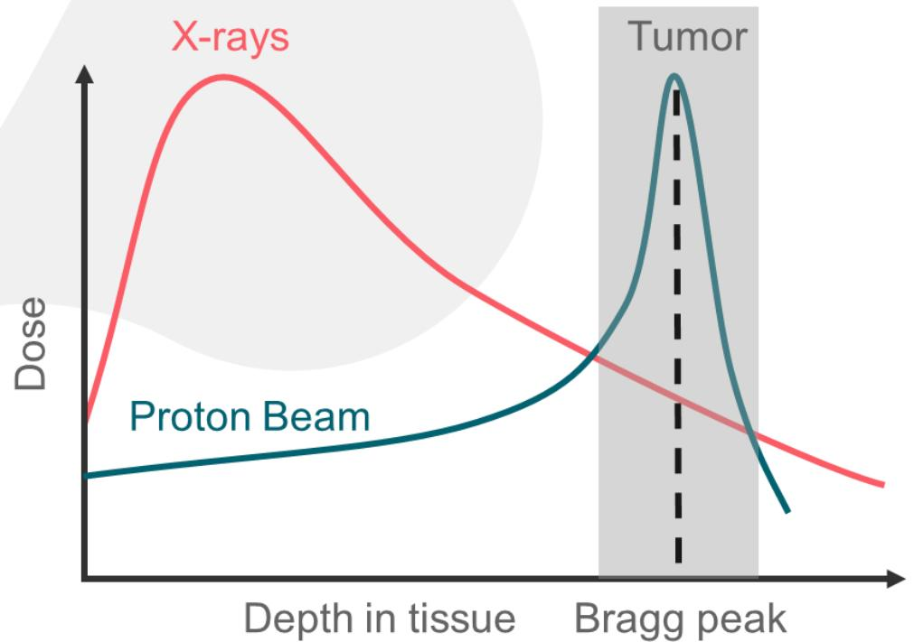
Difference between X-rays and a proton beam for medical use
