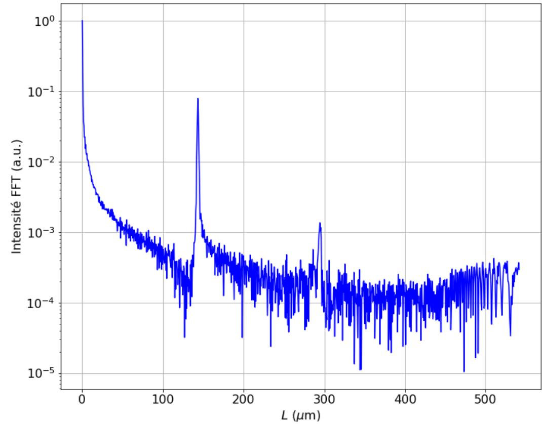
Raw data from spectrometer and fast Fourier transform to get the thickness
