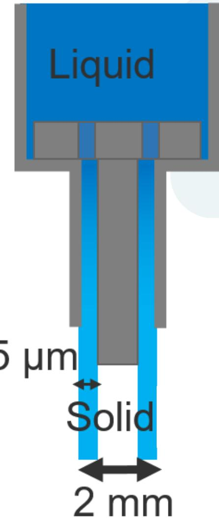
Solid methane target with an adiabatic expansion process
