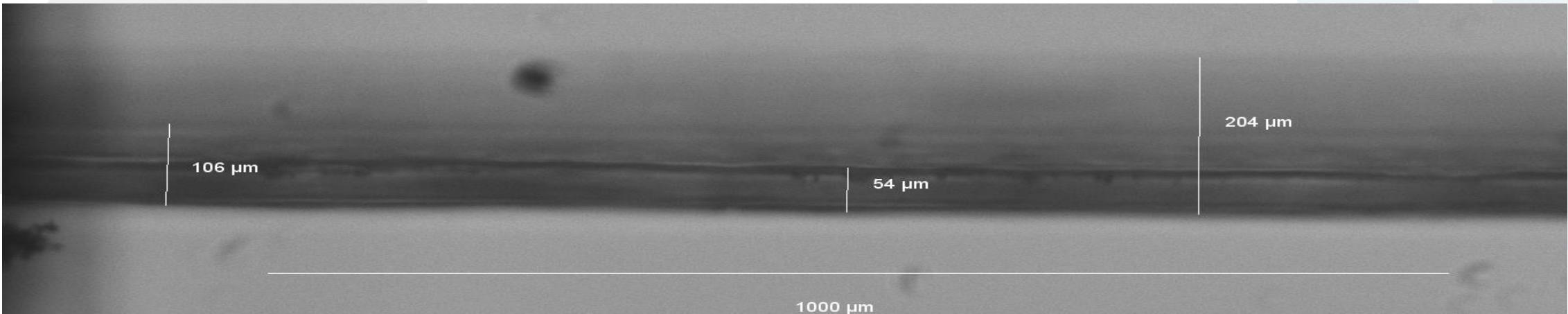
Target thickness observation with long distance microscope Questar QM100
