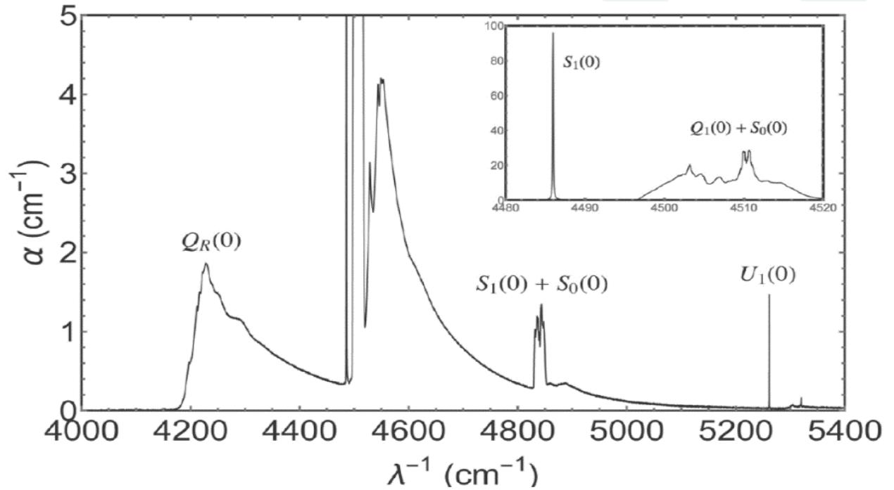
Absorption spectrum of solid hydrogen in infrared range. Peak of absorption at 2.23  $\mu\text{m}$
