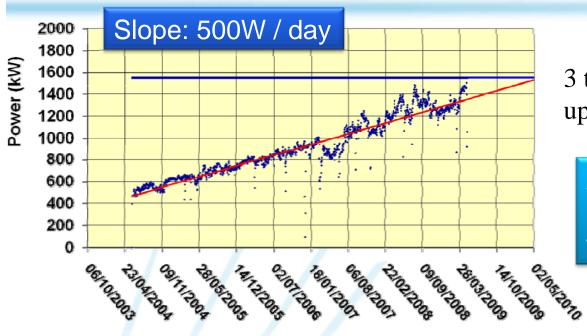
3 transformers: 1550 kW recently upgraded to 3000 kW
