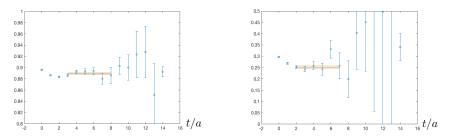
Typical fits used to extract the reduced matrix element (here  $p = 2\pi/L \cdot 2$  and z = 4 (LHS) and  $p = 2\pi/L \cdot 3$  and z = 8 (RHS)). The average  $\chi^2$  per degree of freedom was  $\mathcal{O}(1)$ . All fits are performed with the full covariance matrix and the error bars are determined with the jackknife method.
