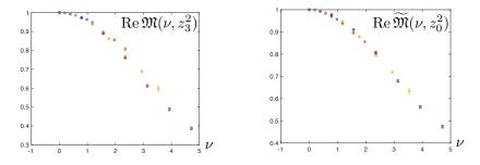
The ratio  $\mathfrak{M}(\nu, z_3^2)$  for for  $z_3/a = 1, 2, 3$ , and 4. **LHS:** Data before evolution. **RHS:** Data after evolution. The reduction in scatter indicates that evolution collapses all data to the same universal curve.
