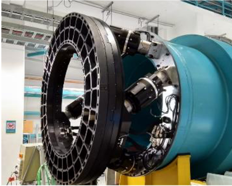
Camera rotator / Camera cable wrap integration
