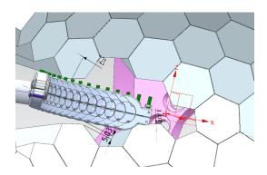
Mechanical clashes with beamline clamp up ~ 35 deg in high-efficiency configuration
