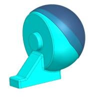
Scattering chamber made of two shells Outer radius 170 mm Thickness 2 mm
