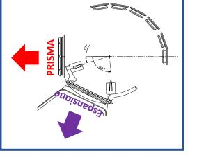
Location of the beamdumps inside the scattering chamber up to 45 deg, at ~80 mm distance from target
