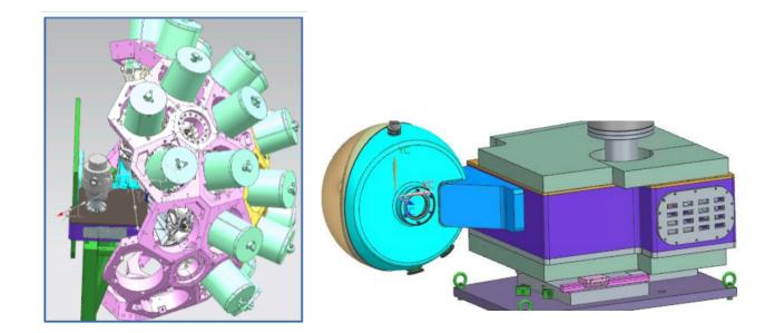
Detailed study of shielding of the expansion chamber to reduce background from beam dumps → See F.Crespi
