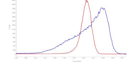
Detector annealing by detector group not satisfying, high yield of broken detectors due to leakage current.
