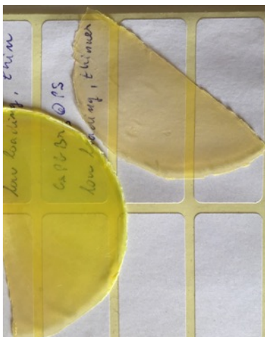
CsPbBr 3 nanocrystals imbedded in polystyrene
