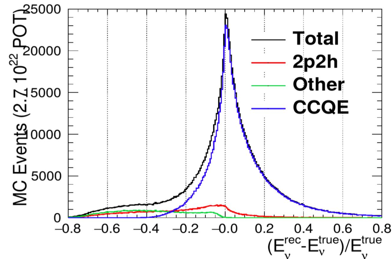
Different interaction processes combined with nuclear effects and not-perfect detectors can introduce a large smearing in  $\nu$  energy reconstruction
