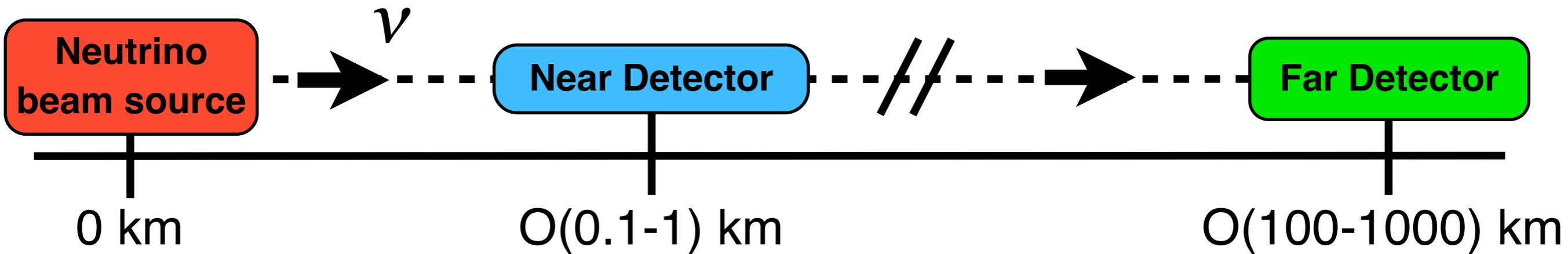
$$N(E_\nu) = \int \underbrace{\Phi(E_\nu, t)}_{\text{Flux}} \times \underbrace{\sigma(E_\nu)}_{\text{Cross Section}} \times \underbrace{R_{det}(E_\nu, \sigma(E_\nu), \vec{r})}_{\text{Detector Response}} \times \underbrace{P_{osc}(E_\nu)}_{\text{Oscillation Probability}}$$
