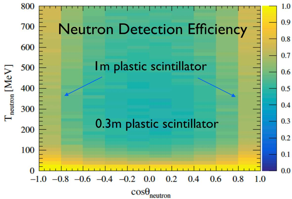
High content of light nuclei ( $\text{C}_8\text{H}_8$ ) ensures high neutron detection efficiency
