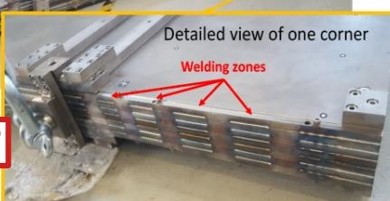
Electron beam welding
