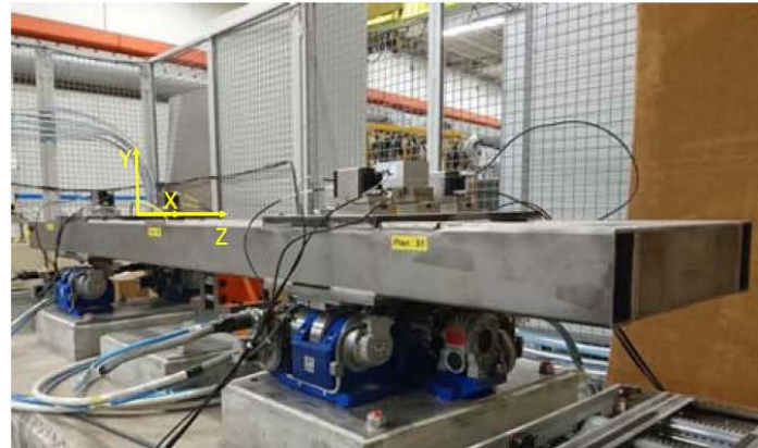
CLIC : Type 4 MBQ and stabilization system mounted on cam movers (left) and test setup including ZCMs, follower girder and local coordinate system (right).
