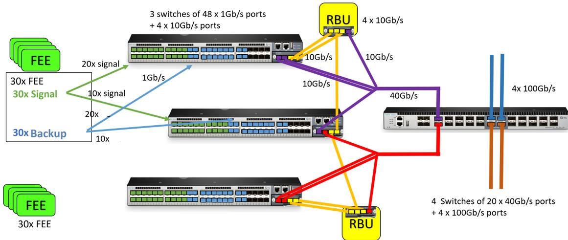
Figure 2: Front end wiring scheme showing readout of 60 FEEs via three switches[centre] ( $\frac{1}{40}th$  of full detector) and one of 4 switches [right] which provide the redundant network for the front end data rerouting
