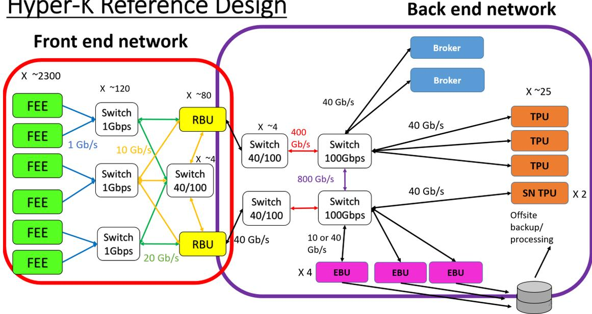
Figure 1: Network reference diagram of the DAQ system.
