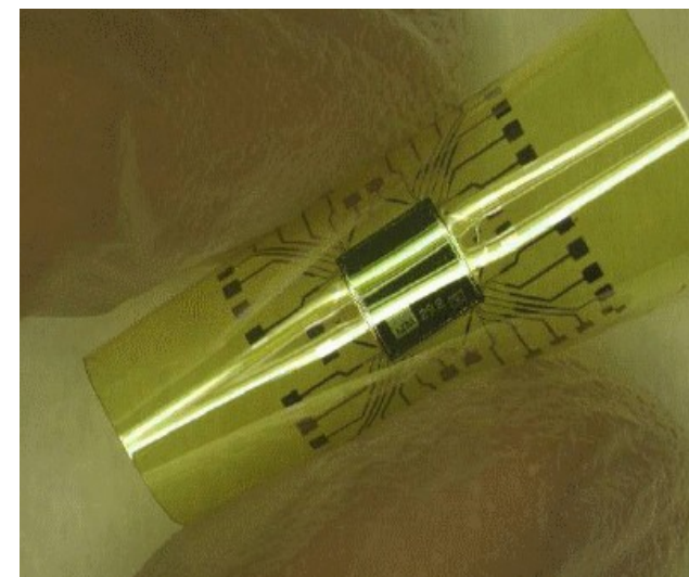
Fully functional microprocessor chip in flexible plastic envelope. *Courtesy of Piet De Moor, IMEC, Belgium
