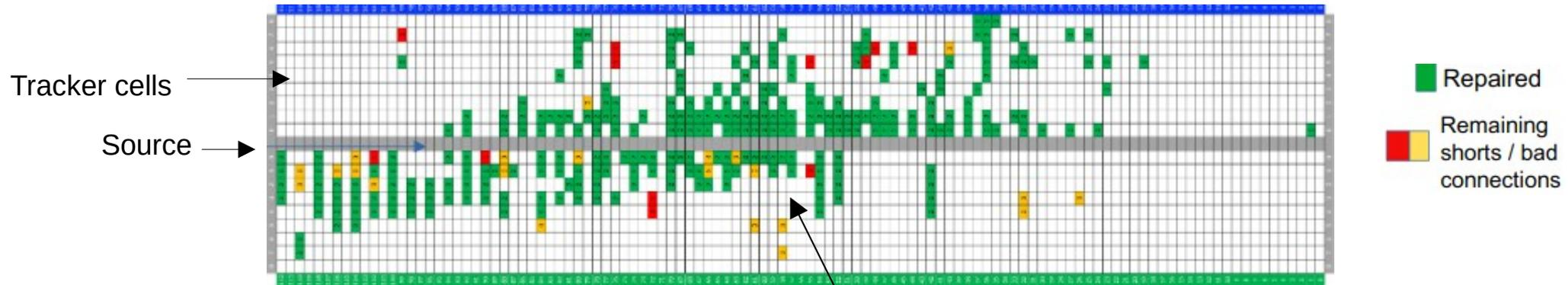
Most short circuits were near the source foils
