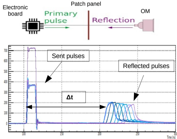
**Reflectometry tests** to test signal attenuation and time delays between PMT channels using electronics generated pulses
