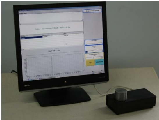
Dosage calibrator for nuclear medicine radio-pharmaceuticals
