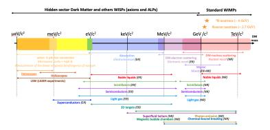
Main techniques used for direct detection of WIMPs (Weakly Interacting Massive Particles, *e.g.* SUSY, KK particles) or WISPs (Weakly Interacting Slim – or Sub-eV – Particles, *e.g.* axions, ALPs, particles from hidden sector), with masses from  $\mu$ eV/c<sup>2</sup> to TeV/c<sup>2</sup>.
