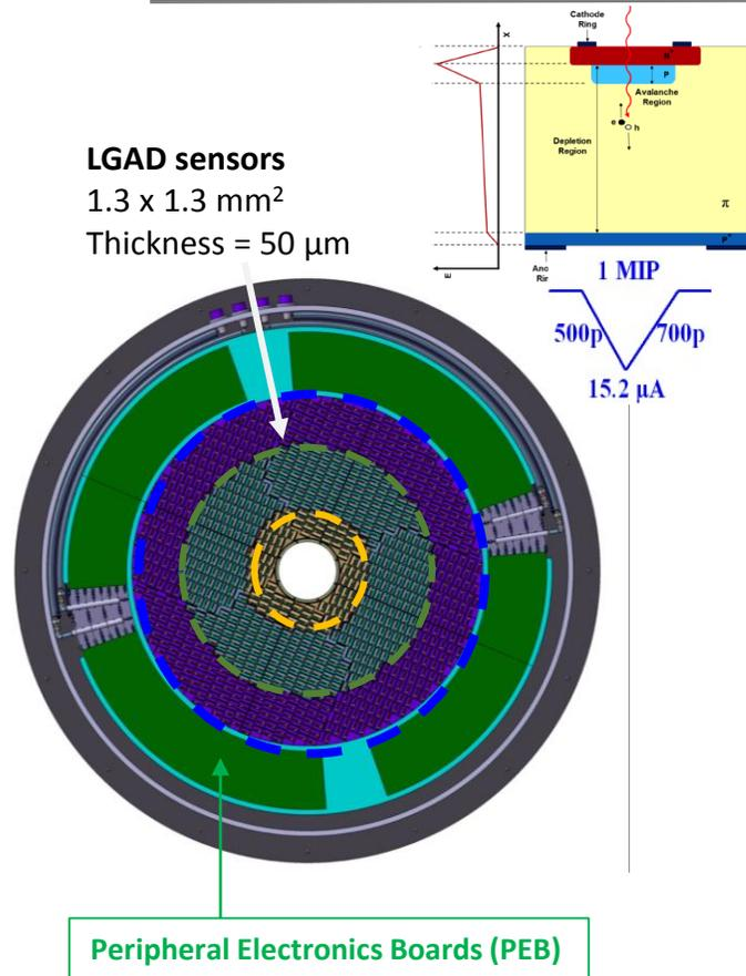
**Active area:** LGAD sensor (450 PADs of 1.3 x 1.3 mm<sup>2</sup>) bump-bonded onto 2 ASICs (225 channels/ASIC)
